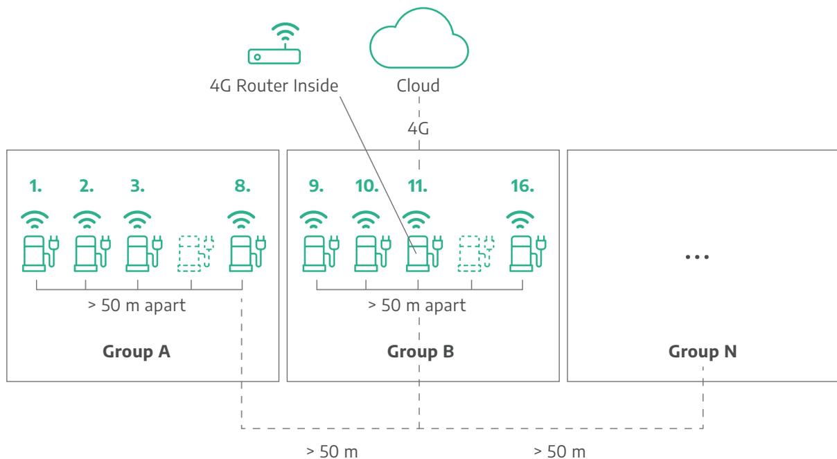
A 4G router is recommended to be installed at the center of all chargers or at a position with the best 4G signal coverage. The 4G router could be supplied by EN+ and it can be installed inside the charger. To keep a stable WiFi connection, the distance between 4G router and the nearest charger should be less than 50 meter. If there are walls or obstacles in between, the distance should be kept less than 20 meter. Same requirement for the distance between two nearby chargers.
